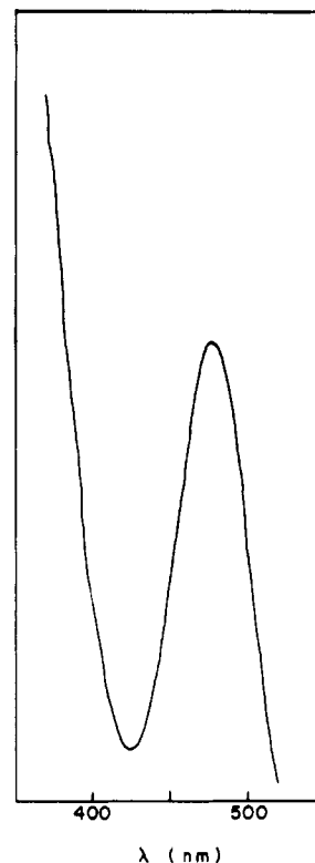
Figure 4. Visible spectrum of the [\text{W}_3\text{O}_2(\text{O}_2\text{CC}_6\text{H}_5)_6(\text{H}_2\text{O})_3]^{2+} ion. The band maximum is at 475 nm with \epsilon = 1080 \text{ M}^{-1} \text{cm}^{-1} .
